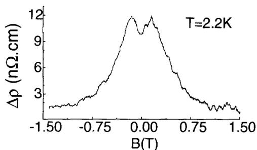
Figure 4. Magnetoresistance of 4 simultaneously contacted Ni nanowires in parallel measured at  $T = 2.2$  with the magnetic field  $B$  directed  $\perp$  to the Ni nanowire.
