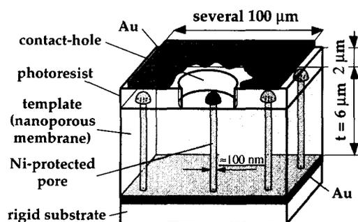
Figure 1. Schematic (not to scale) showing a completely structured device before the dissolution of the Ni in the pore selected by the contact hole.
